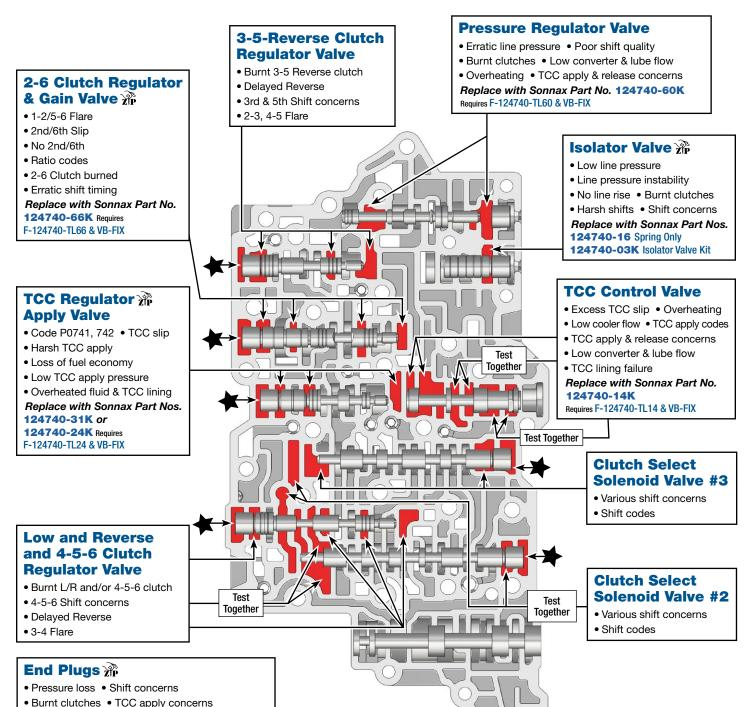
**NOTE:** Vacuum test end plugs at outboard port while sealing
